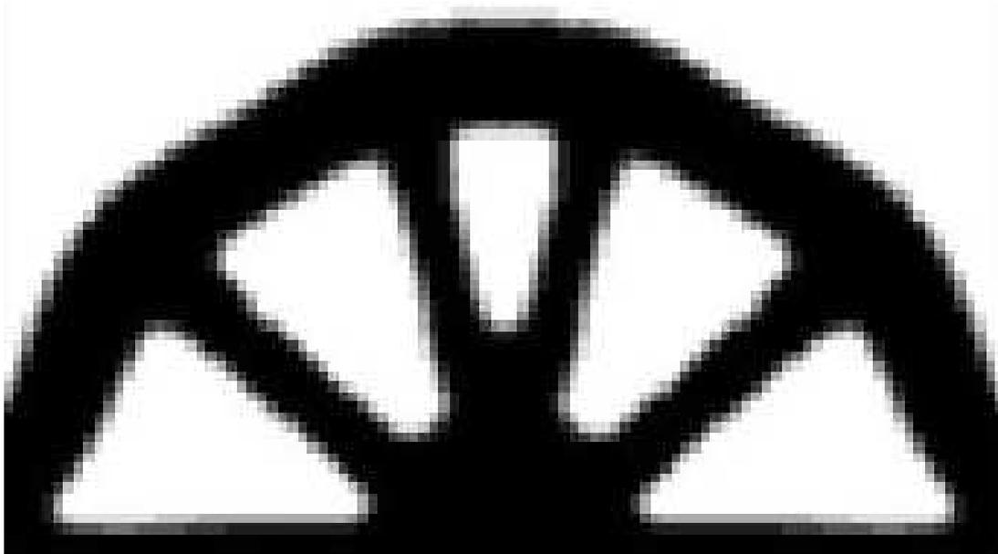
Figure 2: MBB beam optimized for the compliance with an additional constraint over the maximum thickness of the shape
