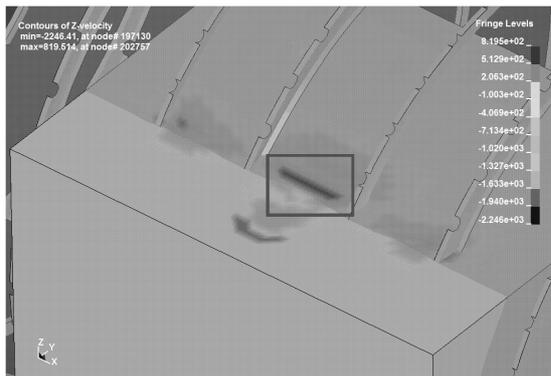
Figure 5: The Euler mesh – non-physical disturbance of the fluid
