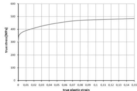
Figure 2: AL2024-T3 stress-strain characteristic [1]
