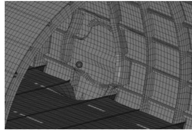
Figure 3: Fuselage deformation (between frames;  $t = 10ms$ )
