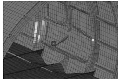
Figure 4: Fuselage deformation (opposite to a frame;  $t = 10ms$ )
