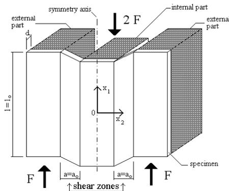
Fig. 3. The scheme of shear device constructed by W.K. Nowacki [4].
