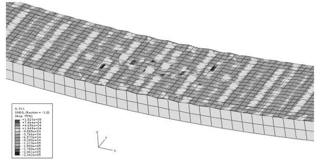
Figure 1: Distribution of normal stress in panel with flat facings
