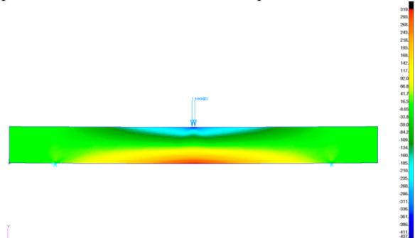
Figure 4. The stress distribution in specimen
