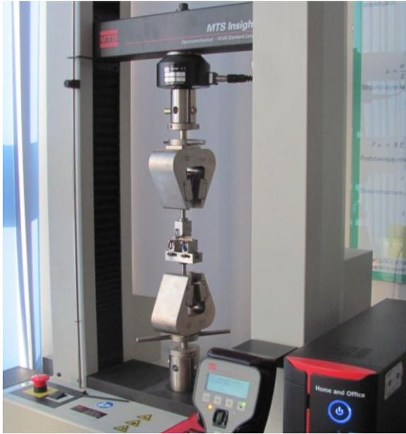
Figure 1: The setup of the three-point bending test
