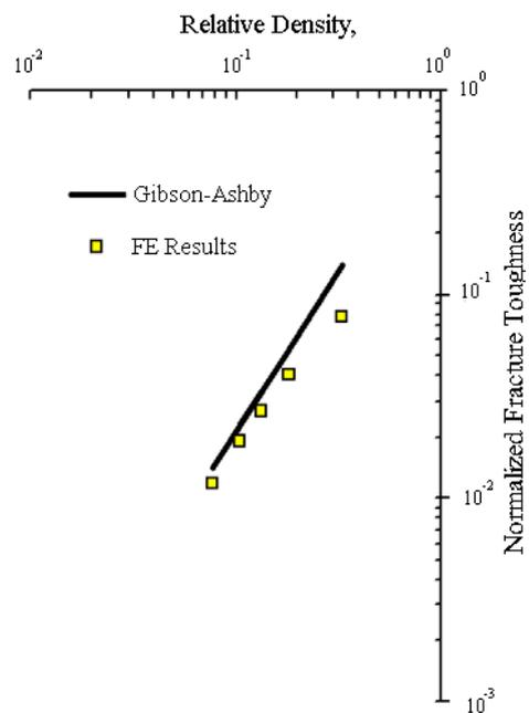
Figure 7: Normalized Fracture Toughness versus Relative Density
