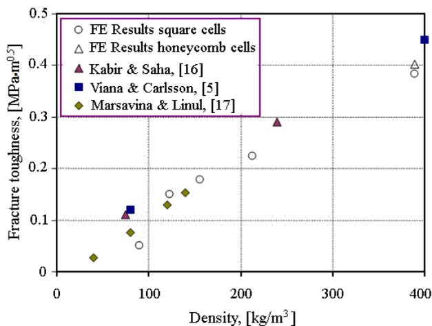
Figure 8: Comparison of estimated Mode I fracture toughness by FE micromechanical model and experimental data
