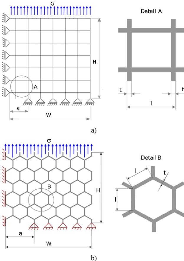
Figure 1: Micromechanical model dimensions and boundary conditions: a) rectangular cells, b) honeycomb cells
