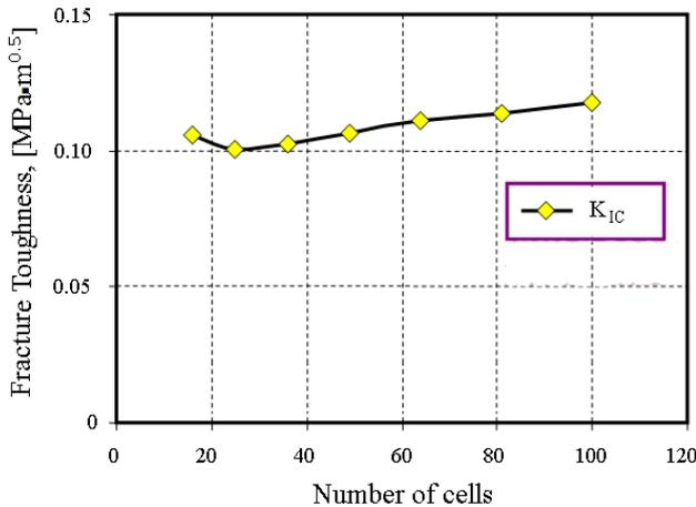
Figure 4: Variation of fracture toughness with number of cells
