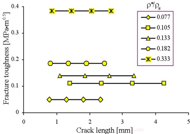
Figure 5: Variation of fracture toughness with crack length
