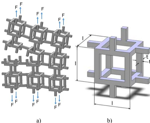
Figure 1: a) Cracked cellular structure; b) cell geometry
