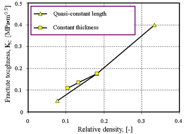
Figure 6: Mode I fracture toughness as a function of relative density for two cases
