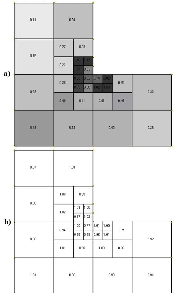
Figure 6: Conforming mesh in Problem B: error estimator  $\eta$  (a), effectivity index  $\theta$  (b).
