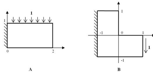
Figure 2: Geometry and loading of test problems
