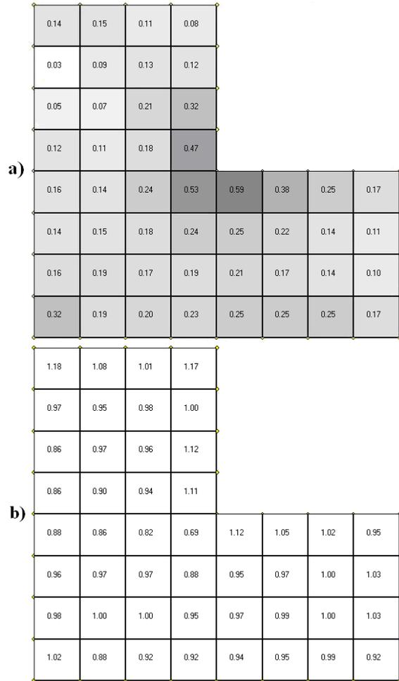
Figure 4: Conforming mesh in Problem B: error estimator  $\eta$  (a), effectivity index  $\theta$  (b).
