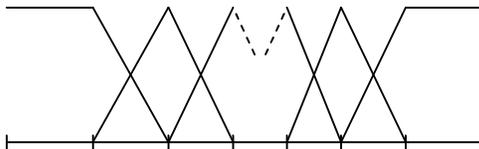
Figure 1: Mortar basis functions
