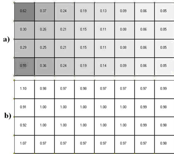
Figure 3: Conforming mesh in Problem A: error estimator  $\eta$  (a), effectivity index  $\theta$  (b).
