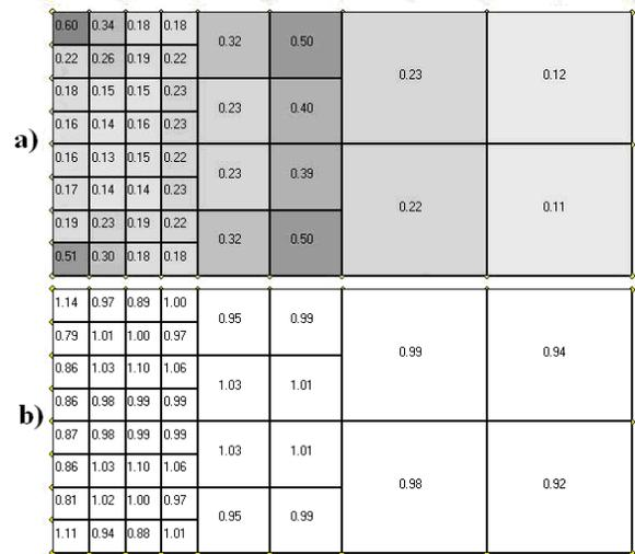
Figure 5: Nonconforming mesh in Problem A: error estimator  $\eta$  (a), effectivity index  $\theta$  (b).
