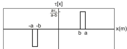
Figure 2: Shear stresses between actuator and plate surface
