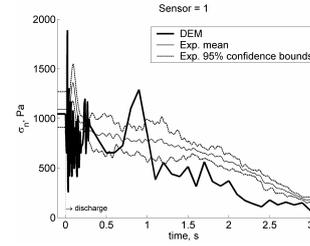
Figure 1: Development of horizontal stress of the wall in discharge.
