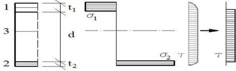
Figure 2: Distribution of normal stresses ( $\sigma_1, \sigma_2$ ) and shear stress ( $\tau$ ) in a sandwich panel with thin flat facings.
