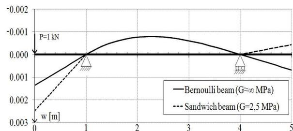
Figure 1: Displacement lines for a sandwich and Bernoulli beam.
