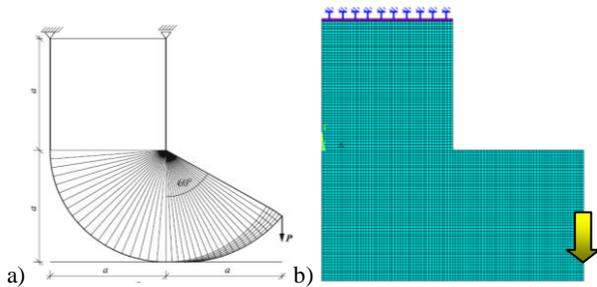
Figure 1: Analytical solution [2] (a) and FE model (b) with displacement boundary conditions and pulsating load ( $R = 0$ )
