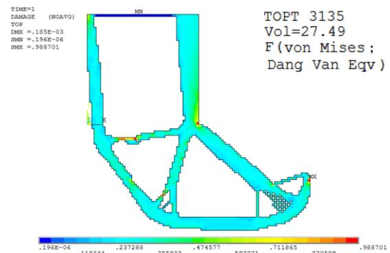
Figure 4: The topology optimization result for multi-constraints (Dang Van and von Mises),  $\bar{g}_a = 1$
