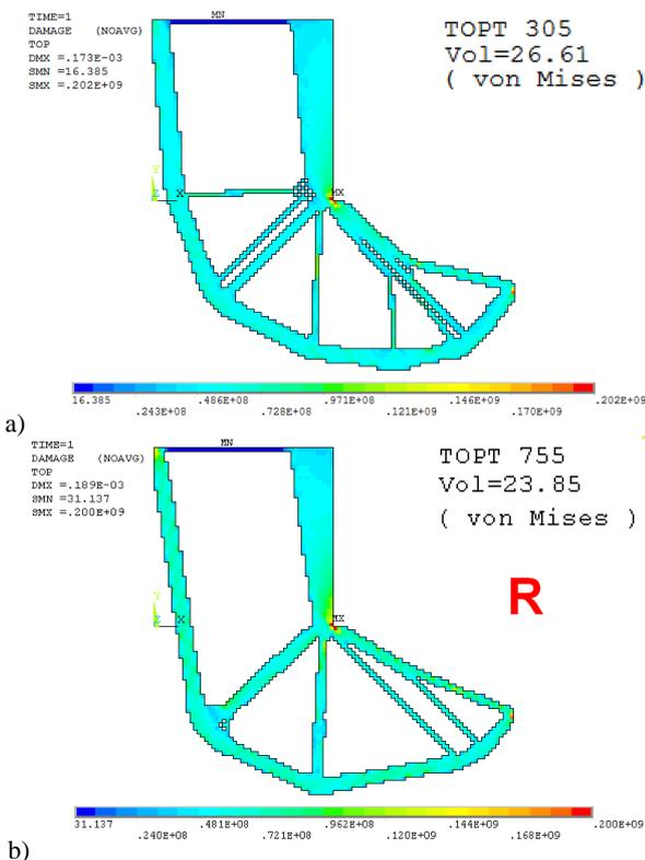
Figure 2: The topology optimization results for von Mises constraint  $\bar{g}_1 = 205$  MPa; start from max. (a) and min. design spaces (reversing) (b)
