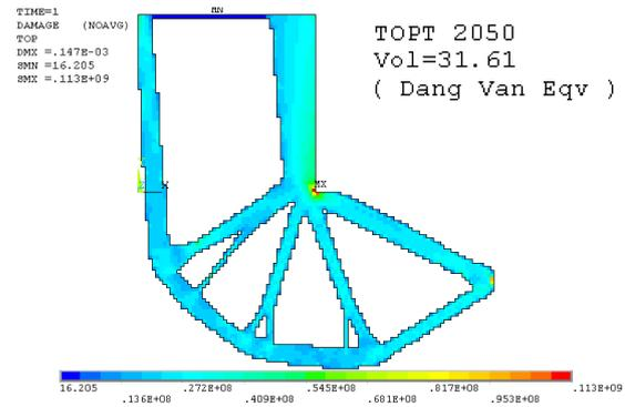
Figure 3: The topology optimization result for Dang Van constraint  $\bar{g}_2 = 114$  MPa (c)
