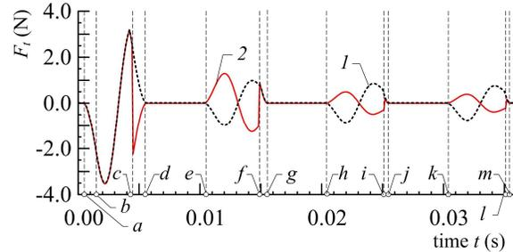
Figure 2: Variation of the tangential force in time for variously calculated direction vectors  $\mathbf{t}$ : 1 -  $\mathbf{t} = \mathbf{F}_t / \|\mathbf{F}_t\|$ ; 2 -  $\mathbf{t} = \delta / \|\delta\|$ .
