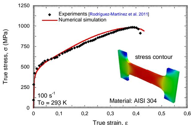
Figure 1. Comparison between numerical predictions of the FE model and experiments at  $100 \text{ s}^{-1}$  and  $T_0=293 \text{ K}$  [6].
