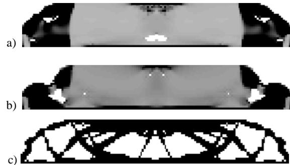
Figure 5: Topologies obtained for  $p=4$  and  $a=0.5$ , using Alg\_1 a), Alg+ b) and Alg- c).
