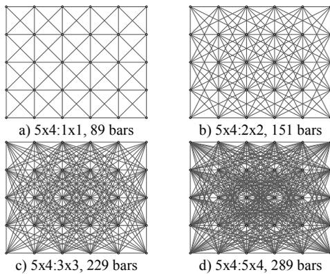
Figure 1: The exemplary successive ground structures
