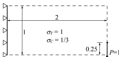
Figure 2: The unsymmetrical cantilever problem from [4]
