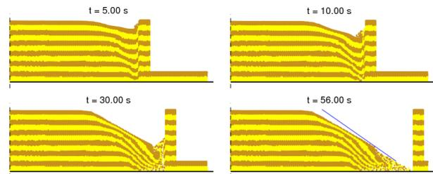
Figure 2: Several phases of the deformation process of the granular material
