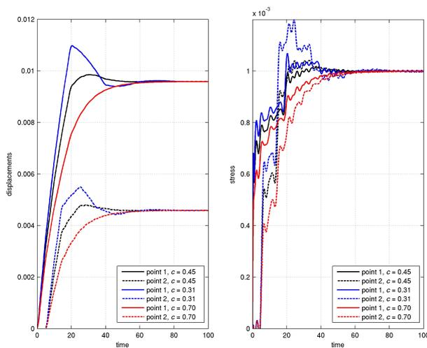
Figure 1: Displacements and stresses as functions of time for three values of the dumping parameter.
