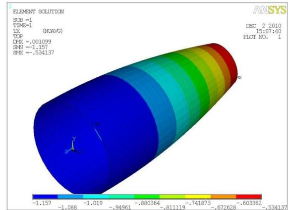
Figure 1: Plot of intensity of circumferential membrane force
