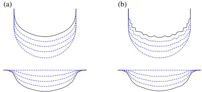
Figure 3: Shape evolution due to wear obtained in (a) 128 and (b) 8 time increments (first-order scheme). The initial and four subsequent shapes are shown, the final configuration is plotted with a solid line (Lengiewicz and Stupkiewicz [2]).
