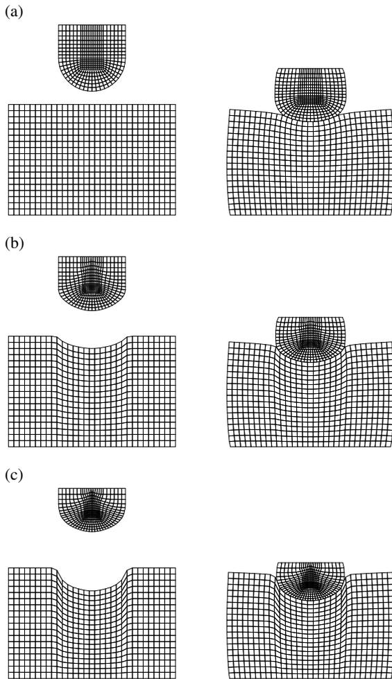
Figure 2: Steady-state pin-on-flat problem (both surfaces wear-off due to out-of-plane motion): undeformed and deformed finite element mesh at three time instants: (a)  $t = 0$ , (b)  $t = T/2$  and (c)  $t = T$  (Lengiewicz and Stupkiewicz [2]).
