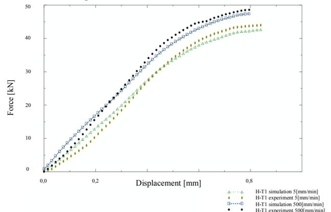
Figure 5: Comparison of different test speeds for simulation and experiment after 40 H-T cycling
