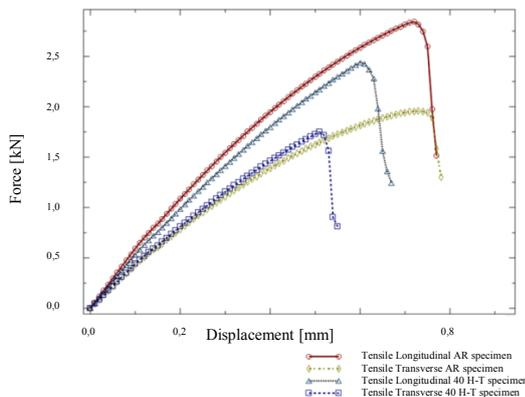
Figure 3: Comparison for AR material and specimens after 40 H-T cycling for tensile test
