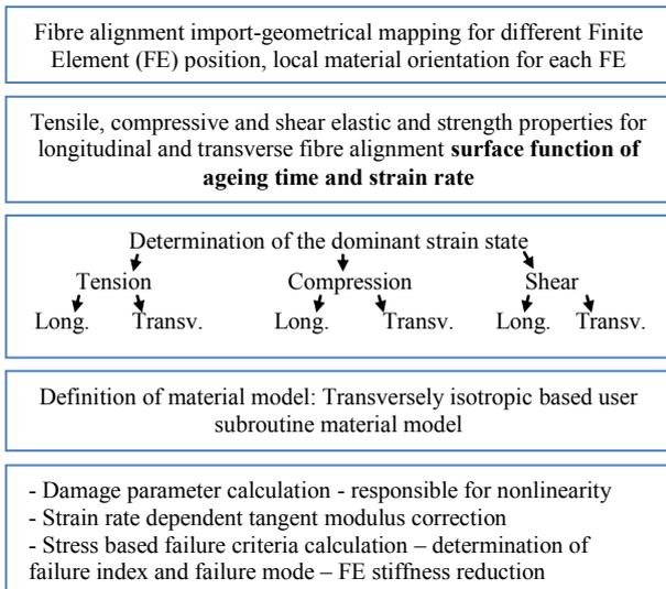
Figure 2: Proposed computation diagram
