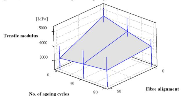
Figure 1: Surface plot of tensile modulus vs. ageing cycles and fibre alignment (0-Longitudinal, 90-Transverse fibre alignment)
