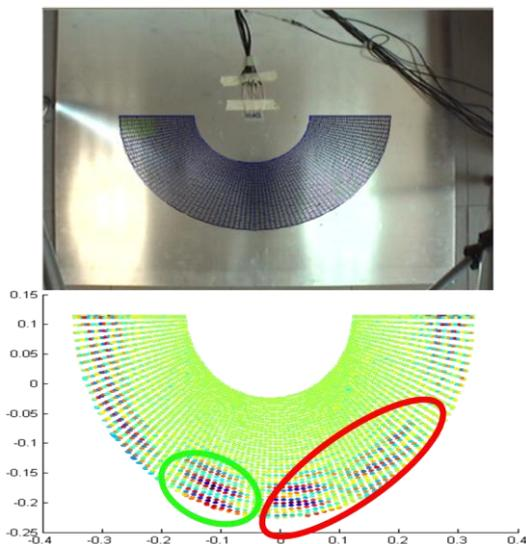
Figure 2: Experimental setup and the results obtained by using laser vibrometer
