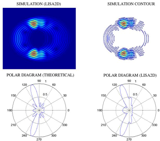
Figure 3: Simulation results for damaged array of transducers
