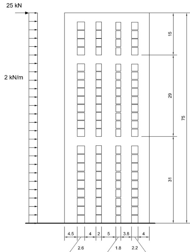
Figure 1. Example 1: Plane shear wall with three stiffening beams and four rows of openings [1]
