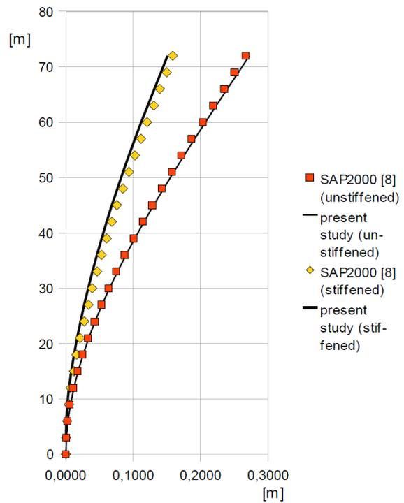
Figure 5. Example 3: Comparison of the lateral displacements in x direction for the unstiffened and stiffened cases
