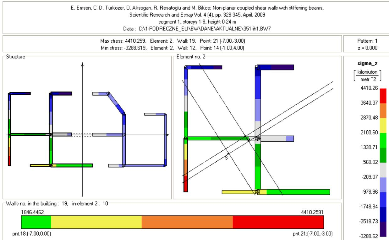
Figure 8. Example 3: Distribution of normal stresses at the base of stiffened shear wall structure
