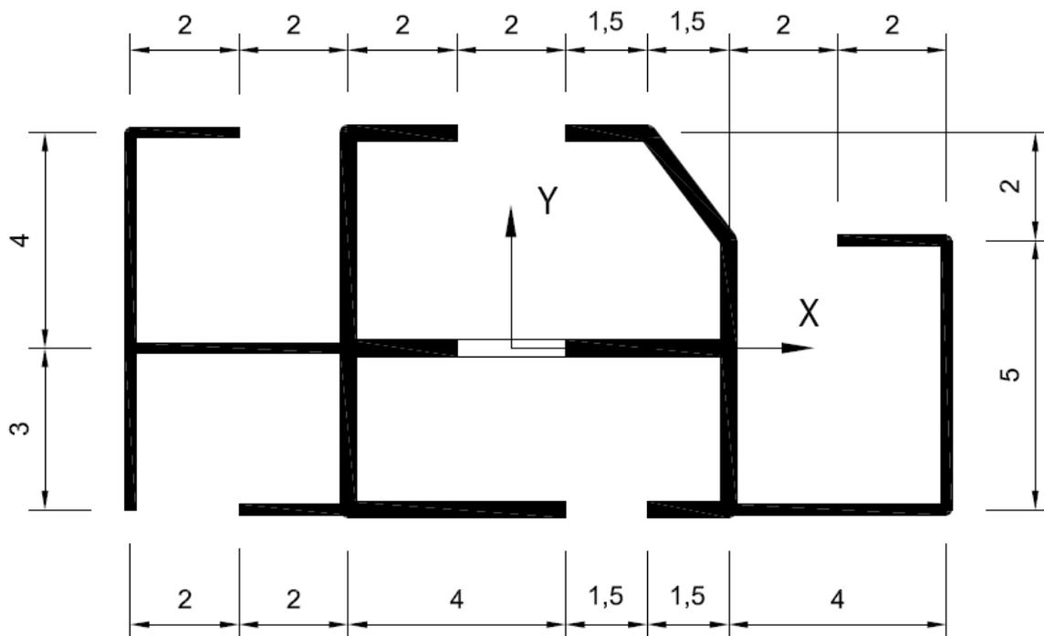
Figure 4. Example 3: Non-planar asymmetrical coupled shear walls with four stiffening beams [8]
