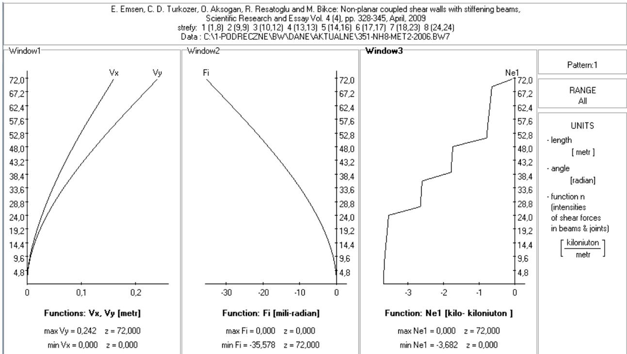
Figure 6. Example 3: Graphs of horizontal displacements and rotations of stiffened structure and normal forces in shear walls
