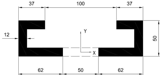
Figure 2. Example 2: The non-planar coupled shear wall Perspex model [7]
