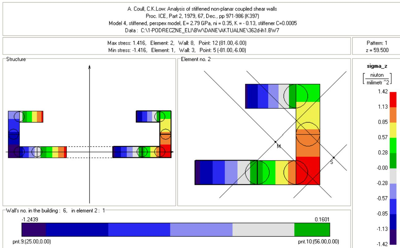
Figure 3. Example 2: The stress distribution in the stiffened non-planar coupled shear wall model at the height  $z = 59.5$  mm
