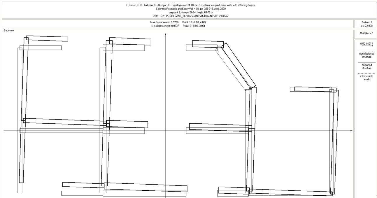
Figure 7. Example 3: Horizontal displacements at the top of stiffened non-planar shear wall structure
