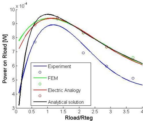
Figure 1: Power harvested by the TEG of a small size (7x7 [mm]) for 3 [K] of temperature difference at the element’s junctions. X-axis presents a ratio of load resistance to generator internal resistance
