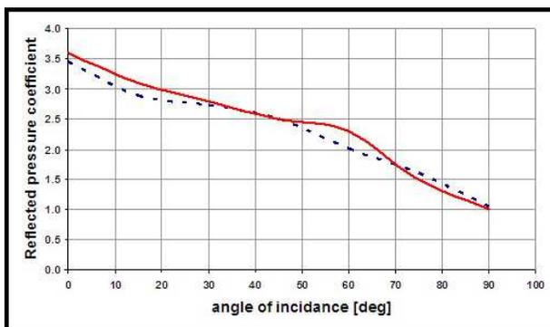
Figure 2: Pressure reflection coefficient compared with codes [3] in function of angle of incidence
