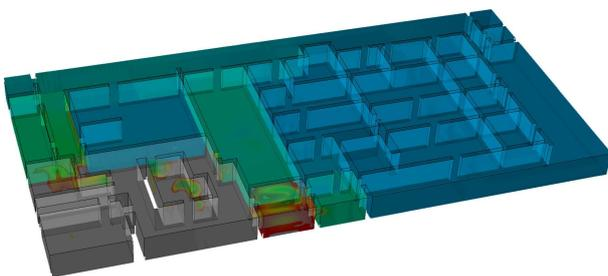
Figure 3: Blast pressure distribution 10ms after detonation
