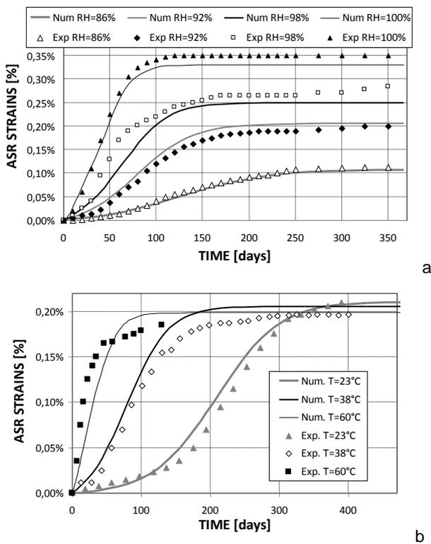
Figure 1. Comparison of the ASR strains obtained from simulations with the experimental data [5]: a) for different values of RH at T=38°C, b) for different values of temperature at RH=92%.
