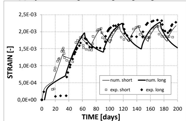
Figure 2. Comparison of the ASR strains obtained from simulations with the experimental data [6].
