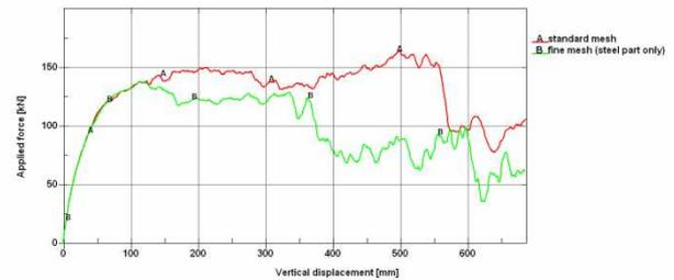
Figure 3: Load versus vertical displacement. Study on mesh resolution
