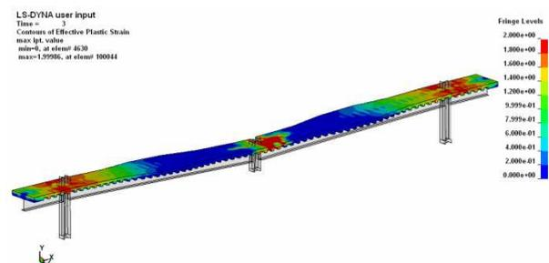
Figure 4: Concentrations of scaled damage measure in the composite slab depicting crack patterns
