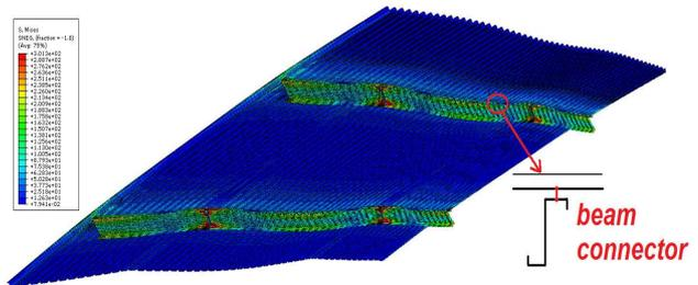
Figure 3: Deformation and effective stress distribution on roof-ing consisting of two zed-purlins and trapezoidal sheet
