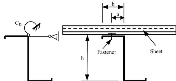
Figure 1: Laterally braced purlin with rotational spring restraint  $C_D$  from sheeting
