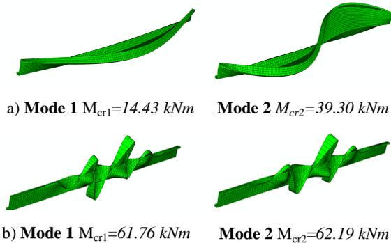
Figure 2: Shapes of buckling mode for purlins: a) without bracings, b) with two bracings
