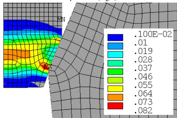
Fig. 1 An example of the plastic strain distribution generated by a single-pass extrusion
