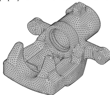
Figure 1: Numerical model of the analyzed disk brake calliper
