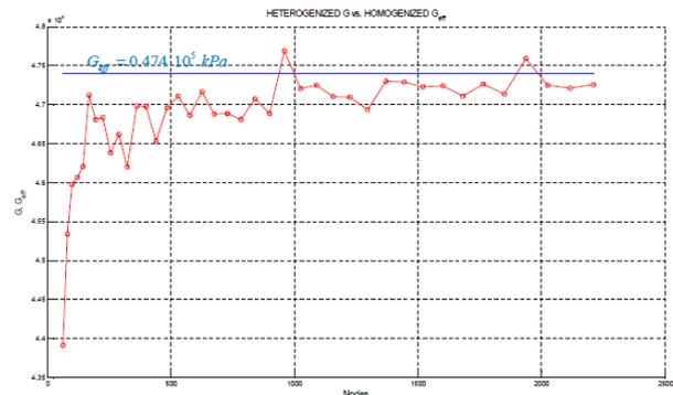
Figure 1: Comparison the average values of the shear modulus ( $G$ ) for the set of more and more denser cloud of nodes with the homogenized one obtained from the RVE analysis.
