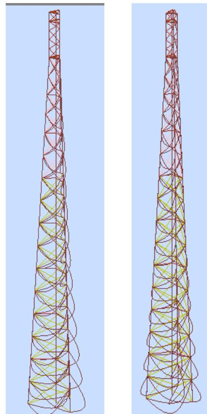
Fig. 2. Deformed configurations of the tower for  $T=-80, 50^\circ\text{C}$
