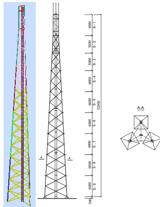
Fig. 1. FEM model of the telecommunication tower
