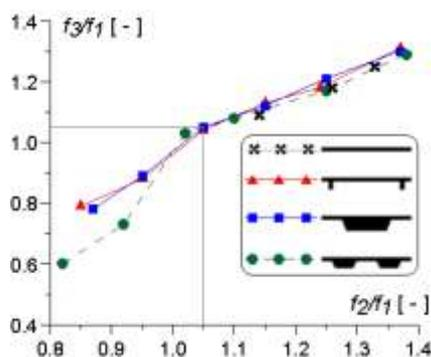
Figure 3: Relation between characteristic frequencies of the aeroelastic system:  $f_1$ ,  $f_2$  – frequency of free vibrations of the system vertical and rotational respectively,  $f_3$  – dominant flutter frequency
