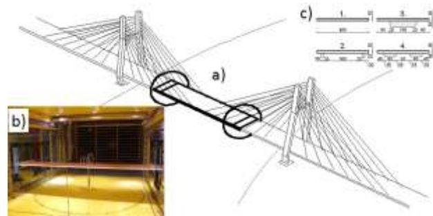
Figure 2: a) central part of a bridge deck under investigation; b) aeroelastic model in a wind tunnel; c) cross-sections of the deck under investigation
