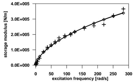
Figure 3 Comparison of the experimentally obtained storage modulus (small crosses) with ones obtained using the three-parameter Maxwell model (solid line with rhombuses) and using the four-parameter Maxwell model (solid line)
