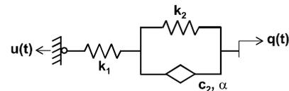
Figure 1: The Kelvin type four-parameter model of VE dampers
