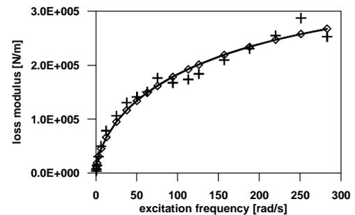
Figure 4 Comparison of the experimentally obtained loss modulus (small crosses) with ones obtained using the three-parameter Maxwell model (solid line with rhombus) and using the four-parameter Maxwell model (solid line)
