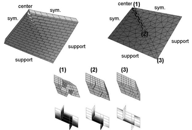
Figure 3: Configuration at peak load of a wall subjected to a central load (displacements magnified by a factor of 500): (top-left) deformed configuration of the complete 3D fine scale computation, (top-right) deformed configuration of the multi-scale shell computation and (bottom) related deformed unit cells.
