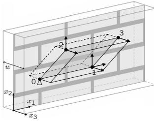
Figure 2: Periodic unit cell for masonry with controlling points
