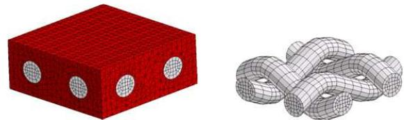
Figure 1: Periodic RVE for a woven composite (left) full RVE mesh with (right) fiber reinforcement discretisation. The unit cell consists of a single period RVE
