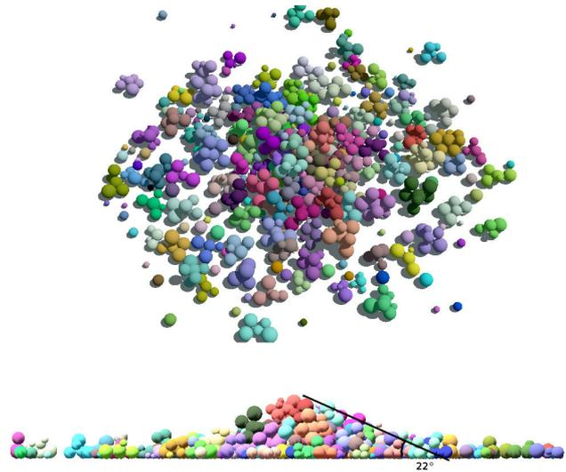
Figure 1: Clumps used in simulation (angle of repose was  $22^\circ$ )
