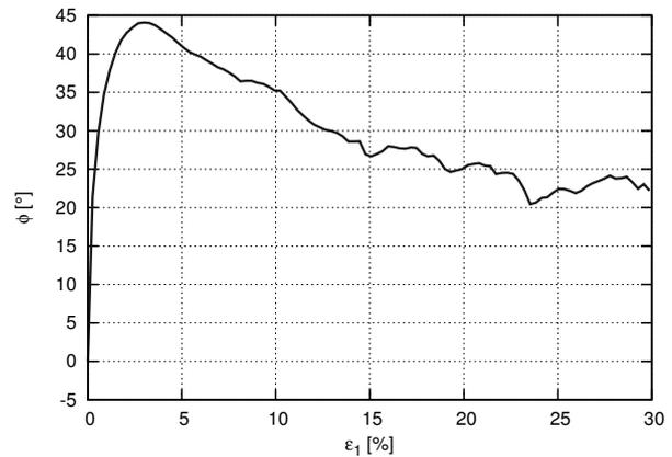
Figure 3: Evolution of global internal friction angle during triaxial test
