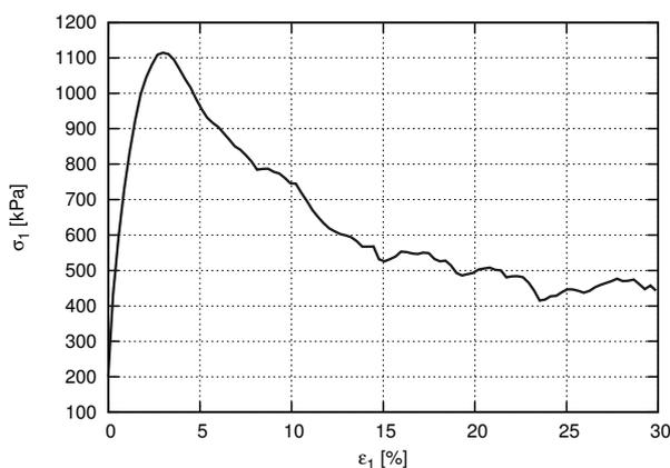
Figure 2: Evolution of vertical normal stress versus vertical normal strain during triaxial test
