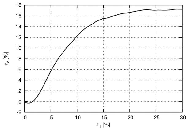
Figure 4: Evolution of volumetric strain versus vertical normal strain during triaxial test
