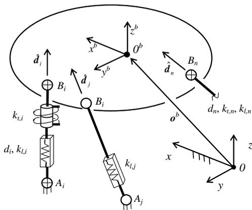
Figure 1: Rigid platform constrained by  $n$ -legs
