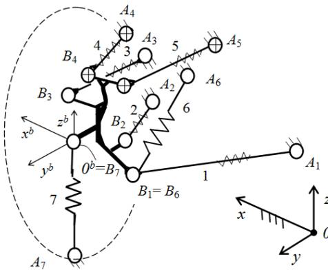
Figure 2: Elastokinematic model of the wheel guiding mechanism with compliant links (no1-5), main spring (no6) and tire (no7)
