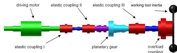
Figure 1: Hybrid mechanical model of the drive system
