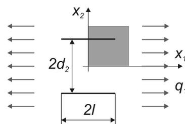
Figure 8: Two rigid fibres in an infinite plate – dimensions and loading
