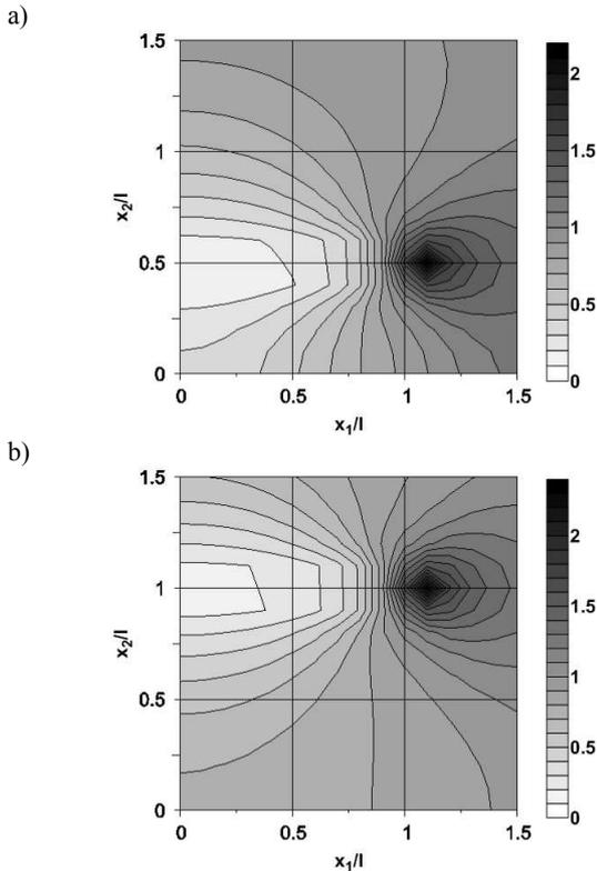
Figure 9. Influence of the distance between two fibres on the stress distribution  $\sigma_{11}/q_1$ : a)  $d_2/l=0.5$ , b)  $d_2/l=1.0$
