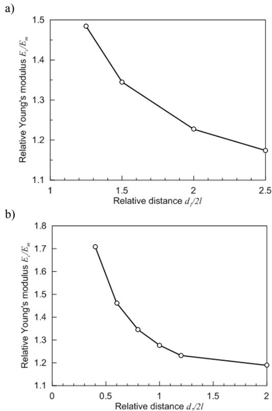
Figure 13. Influence of the distance between the fibres on the relative effective Young modulus  $E_c/E_m$ : a) horizontal distance  $d_1/2l$ , b) vertical distance  $d_2/2l$
