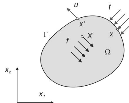
Figure 1. Elastic plate - loading and displacements
