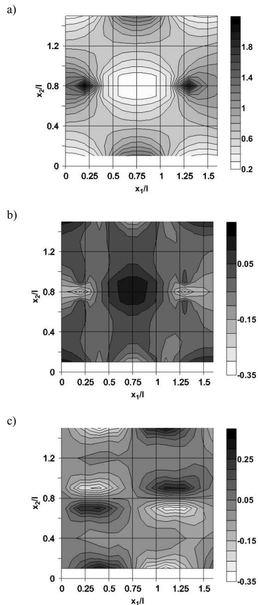
Figure 12. Stress distributions in the matrix: a)  $\sigma_{11}/q_1$ , b)  $\sigma_{22}/q_1$ , c)  $\sigma_{12}/q_1$
