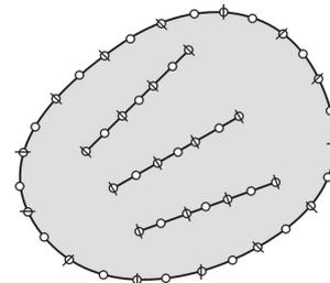
Figure 5. Discretization of the matrix and fibres by quadratic boundary elements
