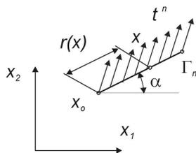
Figure 4. Forces acting on the fibre
