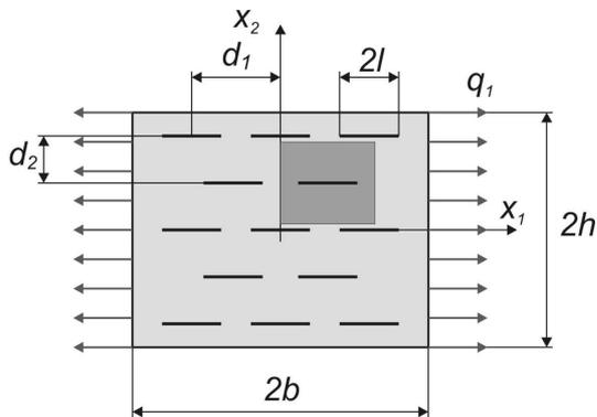
Figure 10: Rigid fibres in a rectangular plate – dimensions and loading
