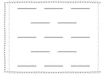
Figure 11. Rigid fibres in a rectangular plate – initial shape (dashed line) and deformed shape (continuous line)
