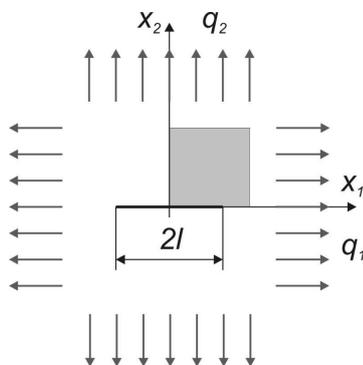
Figure 6: Rigid fibre in an infinite plate – dimensions and loading
