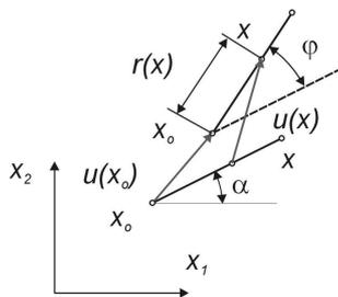
Figure 3. Displacements of the rigid fibre
