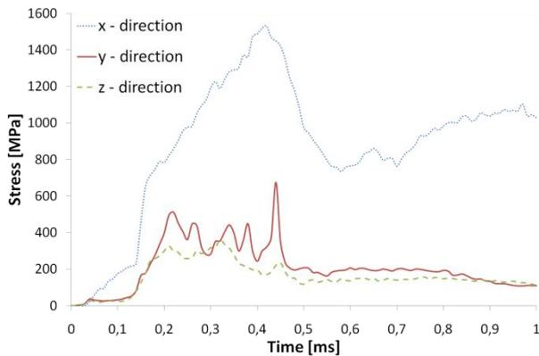
Figure 9: Courses of maximum strains of the middle part of the rod made of St3 steel for the main directions.
