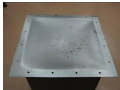
Figure 8: The deformed shape of the base plate
