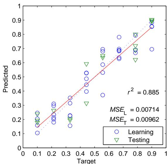
Figure 3: Prediction of the location of damage
