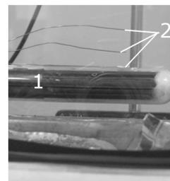
Figure 3: The model of an infant baby (1) with thermocouples (2).
