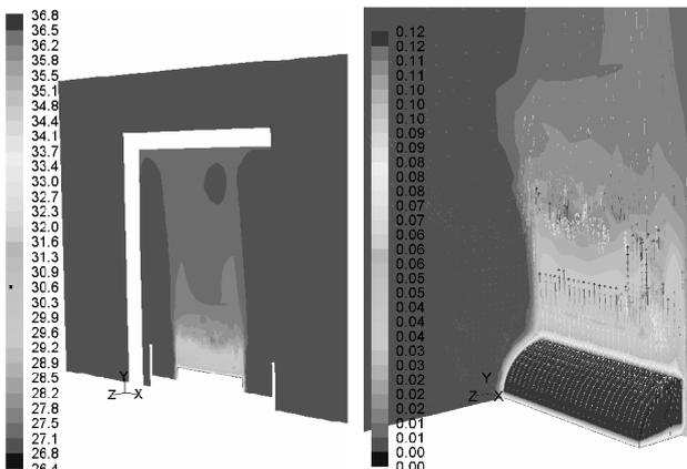
Figure 2: Temperature distribution, whole model °C (left), temperature distribution with vectors m/s (right).
