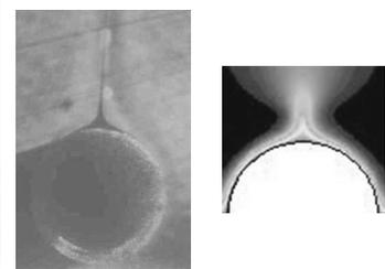
Figure 4: Flow field above infant model. An experimental solution (left), a numerical solution (right).
