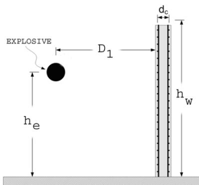
Figure 1: Reinforced concrete blast wall height  $h_w$ , height of burst  $h_e$ , stand-off distance  $D_1$ , wall effective depth  $d_c$  and height  $h_w$ .
