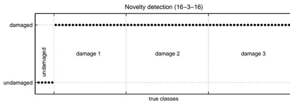
Figure 2: Results of novelty detection applied to aluminum strip - test of NN (16-3-16)
