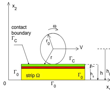
Figure 1: The wheel rolling over the strip.
