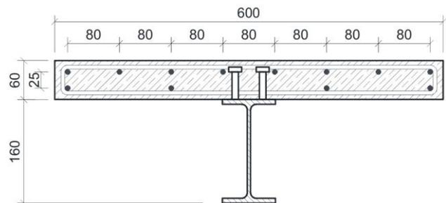
Figure 1: Cross - section of composite beam
