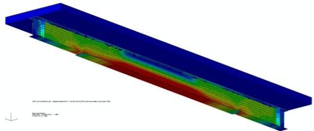
Figure 4: Stress in the beam and in the plate
