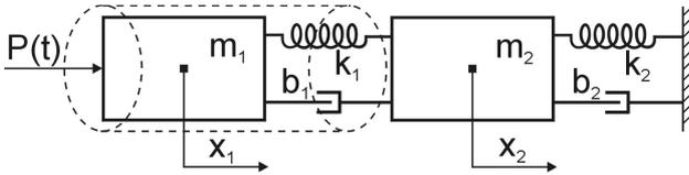
Figure 2: Mechanical system modelling duct with transmission loss frequency-dependent characteristic. Pipe's domain is denoted by dash line
