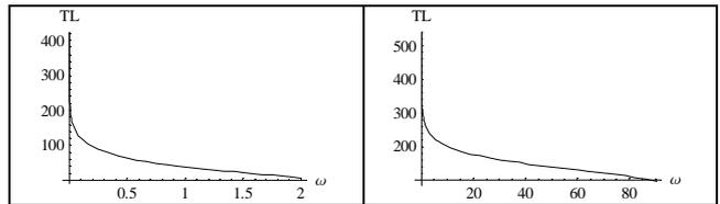
Figure 4: Plot of a transmission loss of mechanical system (left)  $m_1 = 10^{-5}, m_2 = 10^{10}, k_1 = 10^{-1}, k_2 = 10^{11}, b_1 = 0, b_2 = 10$ , (right)  $m_1 = 10^{-5}, m_2 = 10^3, k_1 = 10^{-1}, k_2 = 10^{10}, b_1 = 0, b_2 = 10$
