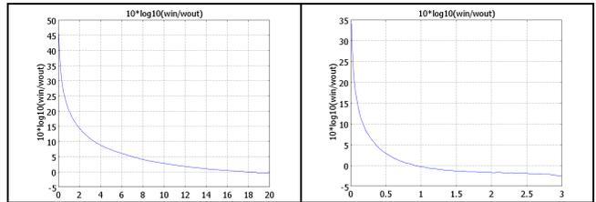
Figure 3: Plot of a transmission loss of pipe with ratio  $r/L$  equals: 0.01 (left) and 0.2 (right)
