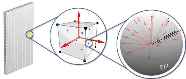
Figure 1: Illustration of the micro-sphere approach: macroscopic boundary value problem (left); particular finite element with integration points (middle); micro-sphere associated with finite number of integrations directions and one-dimensional constitutive law represented by the spring-dashpot device.
