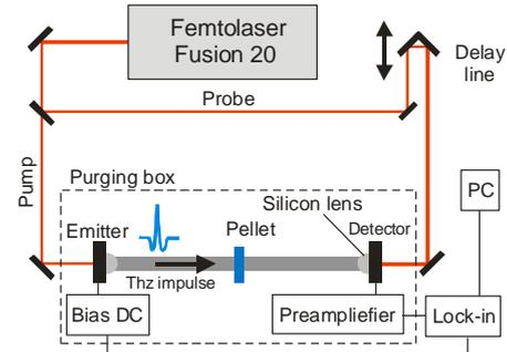
Figure 2. Time Domain Spectrometry setup [2]
