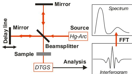
Figure 1. Fourier Transform Infrared Spectroscopy setup [1]
