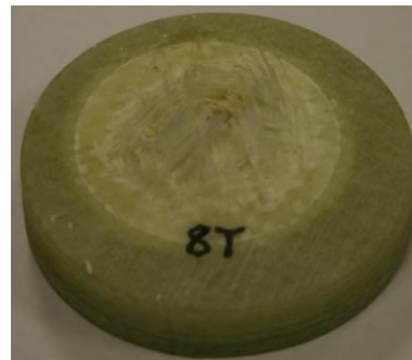
Figure 7. Multilayer glass composite sample shut with the bullet – real photo
