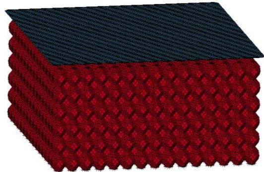
Figure 6. Finite element model of the aluminum foam microstructure
