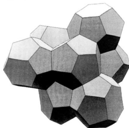
Figure 2: Weaire-Phelan repeatable structure
