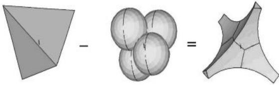
Figure 4. A tetrahedron and spheres to generate a unit cell of a foam [6]
